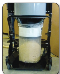
Kit LONGOPAC for the collection of the sucked materials into tubular continuous bag
