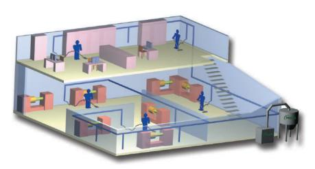
control systems) and **centralized ventilation systems** (such as dust collectors, electro-fans, mobile arms, electrical control panels and piping components).
