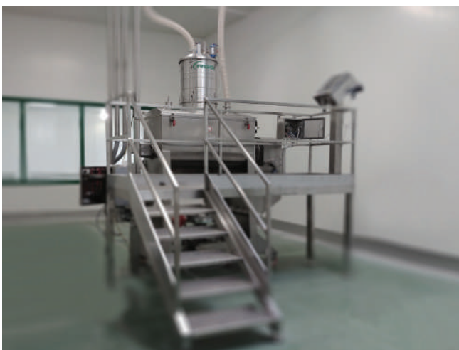
Hopper on mixer for the transport of powders pharmaceutical and nutraceutical.
