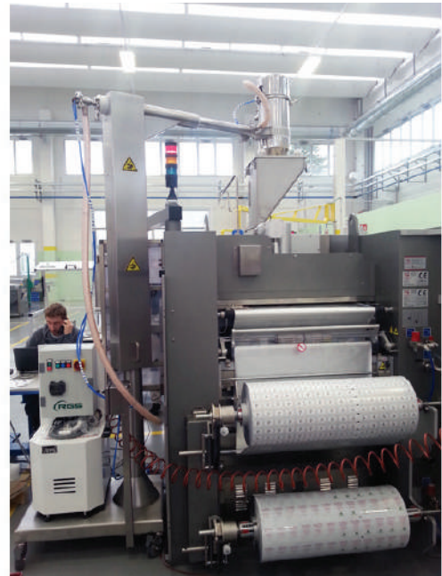
High vacuum conveyor system of pharmaceutical powders with pneumatic lifter to facilitate the positioning of the hopper over the packaging machine.
