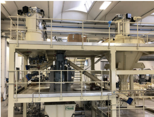
Pneumatic conveying system for tobacco powders, storage in silos and dosage on mixer.
