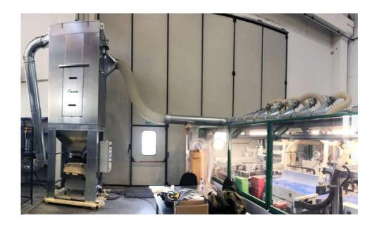
Localised extraction has the task of capturing pollutants as close as possible to the point of production of the pollutants (source) and abating them before they are released into the atmosphere to reduce concentrations to values compatible with environmental protection.
