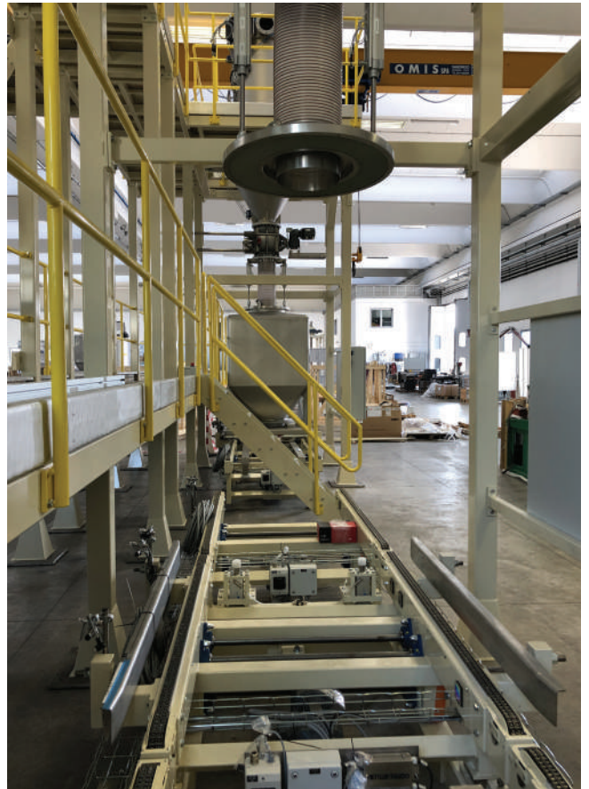
Conveyor system for tobacco powders.
