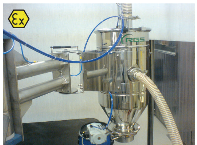
Conveyor system for mixed pharmaceutical powders made of 316L AISI stainless steel with polished finishes in a pharmaceutical industry. System realized in version ATEX for zone 21-22.
