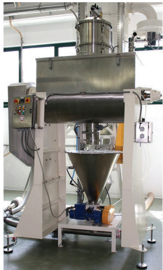
Pharmaceutical mixer working in depression.
