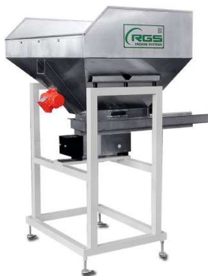
“Square section hopper with vibrating channel”
