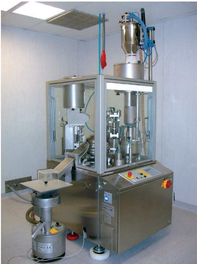
Conveyor system for pharmaceutical blending on an capsule filling machine in a pharmaceutical industry.
