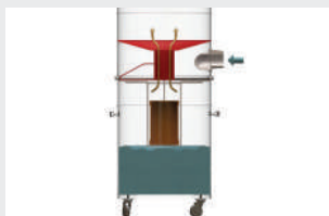
Mechanical float to stop suction
