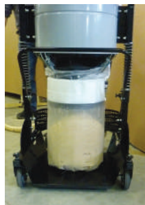
LONGOPAC kit for product discharge in continuous bag
